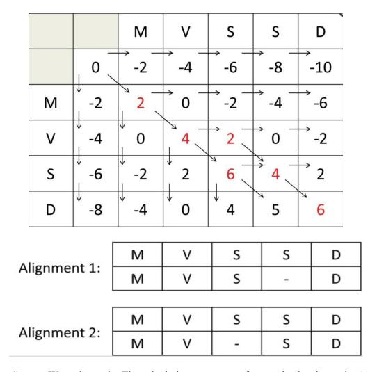
Figure 1 Needleman—Wunsch matrix. The calculation uses scores for match +2, mismatch -1, and gap -2. The arrows show the matrix cell from where the value is generated. Red-coloured cell values show the trace back that creates alignment.
